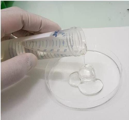
Figure 3. (left) pouring the epoxy slowly in the petri dish. (right) Make sure that you put enough resin to entirely cover the microfluidic device.
