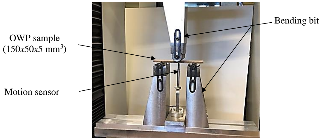
Figure 5: Bending elasticity modulus and strength testing device
