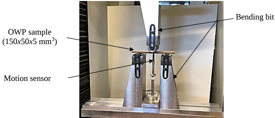
Figure 5: Bending elasticity modulus and strength testing device
