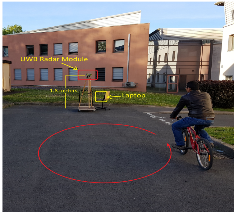
Figure (5.20) Radar setup and an example of experiment where a cyclist moved in front of the radar
