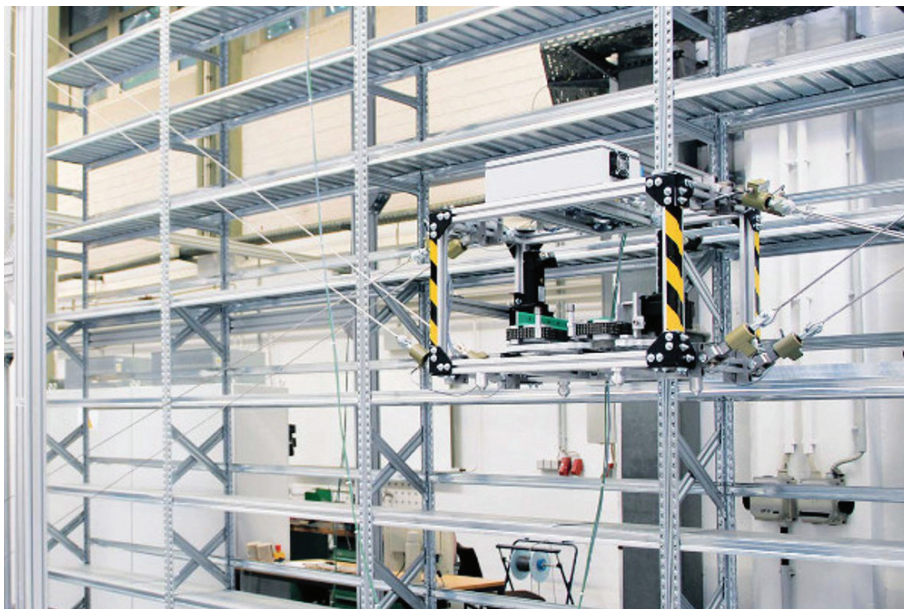
Figure 2.8: CABLAR CDRP prototype developed by University of Duisburg-Essen
