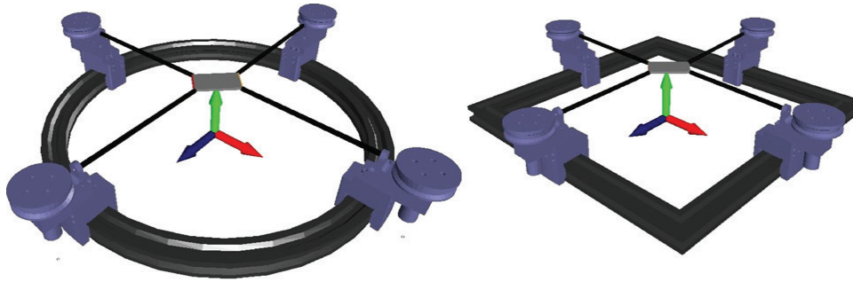
Figure 2.11: CDPRs with base mobility in multi-domain modeling and simulation tools [AAK17]
