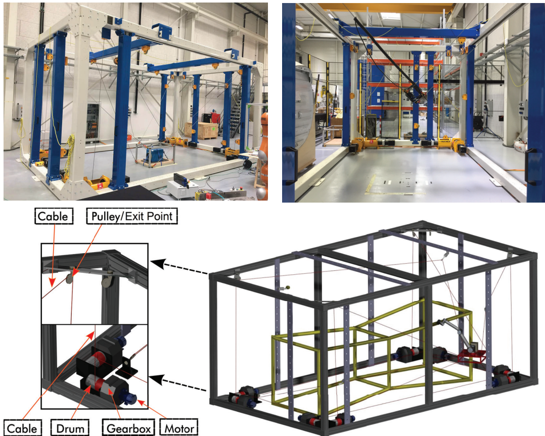
Figure 2.10: CAROCA prototype located at IRT Jules Verne (Technocampus Ocean)
