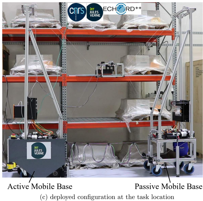
Figure 1.11: FASTKIT working modes
