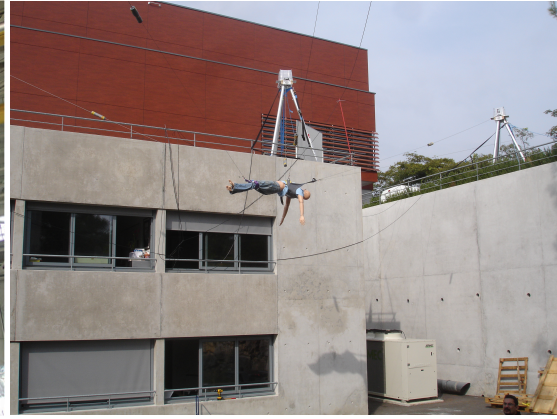
Figure 2.2: MARIONET-CRANE, CDPR for search and rescue operations
