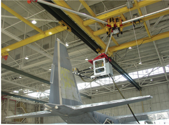
Figure 2.1: NIST RoboCrane painting an aeroplane
