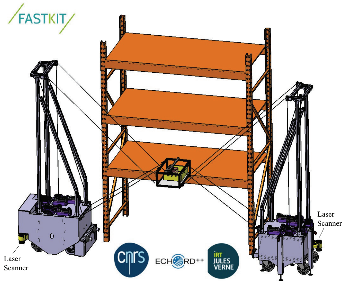
Figure 1.5: FASTKIT concept: A cable-driven parallel robot mounted on two mobile platforms [PRMG + 20]
