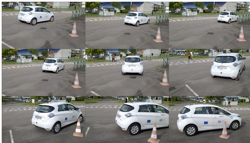
Figure 4.24: Experimental car parking in a parallel spot
