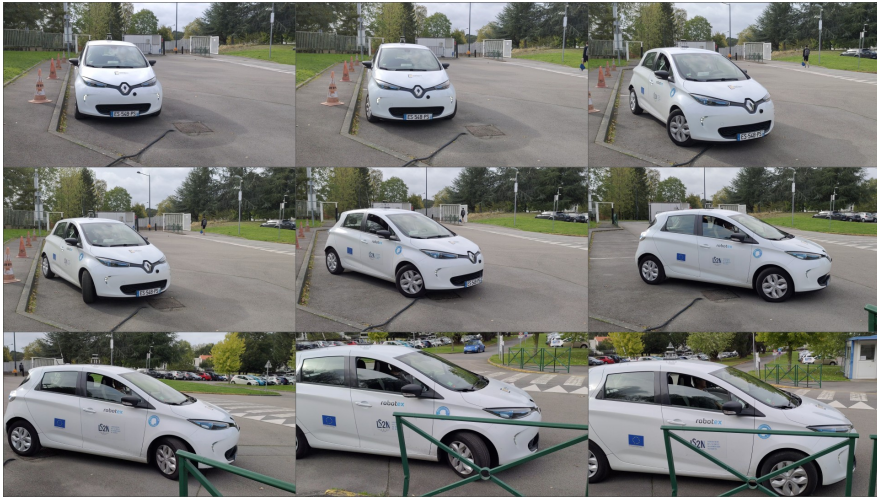
Figure 4.26: Experimental car unparking from a parallel spot
