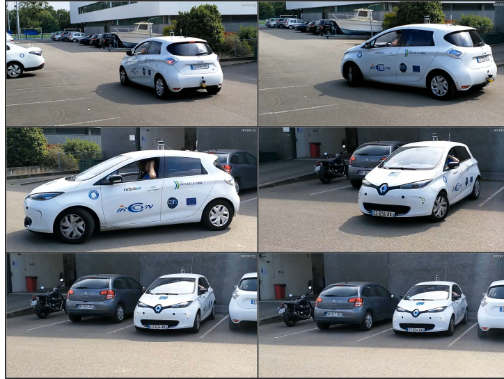
Figure 3.30: Experimental car parking in a perpendicular spot using online feature extraction
