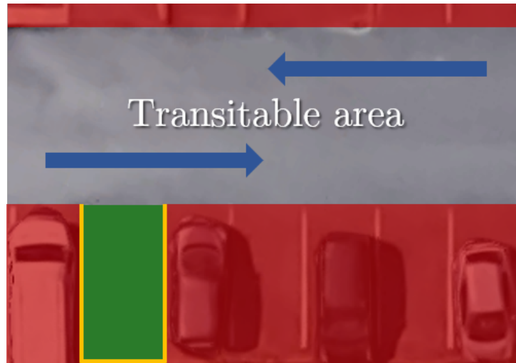
Figure 4.2: Example of a parking environment. The green rectangle denotes the parking spot into which the car should park. Red areas are considered forbidden zones, as such the vehicle should never go into them. Furthermore, it is considered that parking maneuvers can only start inside the transitable area and if no portion of the vehicle is inside any of the forbidden zones while unparking maneuvers can only start if the vehicle is in a parked pose (i.e. inside a parking spot).
