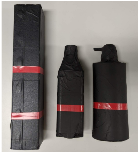
FIGURE 4.3: Distinguishable shape and mass objects used during one-handed handover between human and humanoid co-worker.
