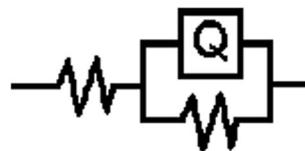
**Fig. 10** Equivalent electrical circuit used for modeling the electrochemical impedance spectra of copper coated by TiO(OH)<sub>2</sub>/MnO<sub>2</sub> composite
