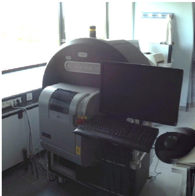
Figure M5 PerkinElmer's Quantum FX microCT Pre-clinical In Vivo Imaging System, Caliper, Life Sciences.
