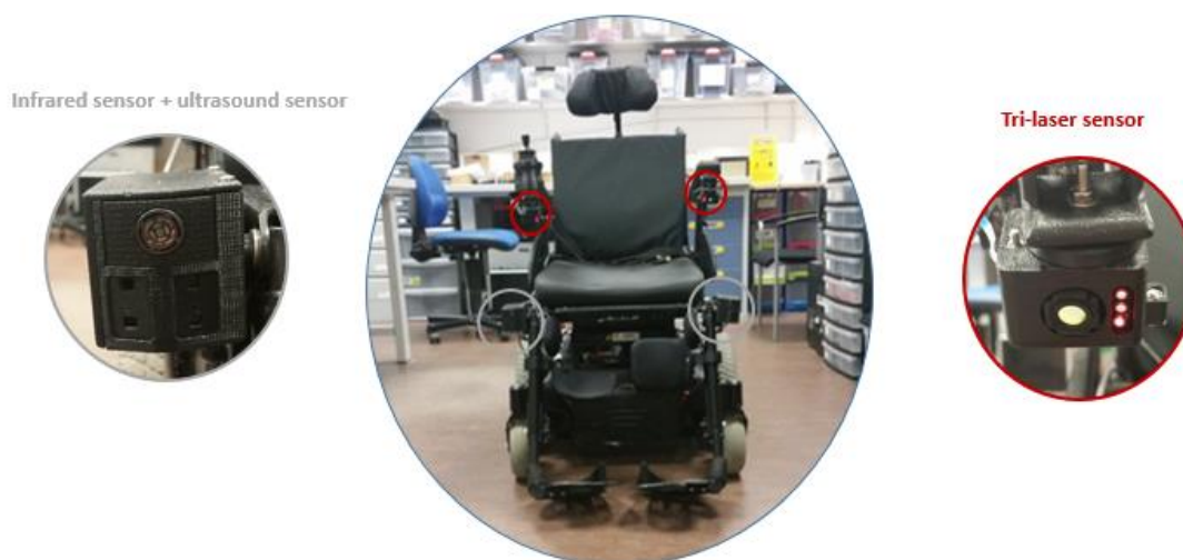
FIGURE V-3 : THE SENSORS USED IN THE CURRENT STATE OF THE AUGMENTED WHEELCHAIR
