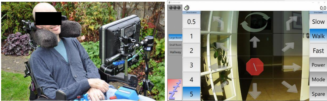
FIGURE II-15 : EYEDRIVOMATIC WHEELCHAIR STEERING SYSTEM. ON THE LEFT A PERSON IS USING THE SYSTEM. ON THE RIGHT, THE SCREEN SHOWS THE USER INTERFACE. 20
