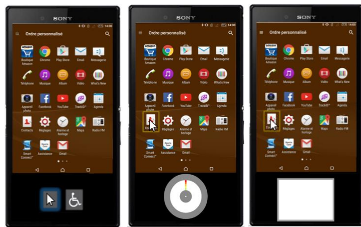
FIGURE VI-11: PHONE INTERFACE ENHANCED BY THE VIRTUAL TACTILE PAD AT THE BOTTOM. ON THE LEFT, THE INTERFACE NO MODE IS SELECTED YET. IN THE CENTER, THE USER HAS SELECTED THE STEERING MODE.
