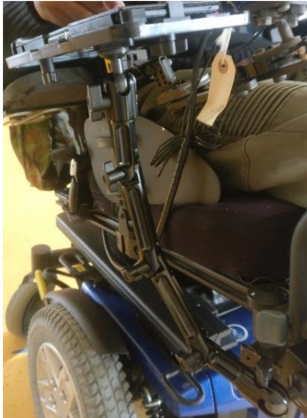
FIGURE IV-1 : THE ARTICULATED FIXATION OF THE TABLET
