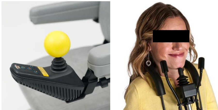
FIGURE II-17 : LEFT: A JOYSTICK WITH A BALL-SHAPED HANDLE 22 RIGHT: A CHIN JOYSTICK 23
