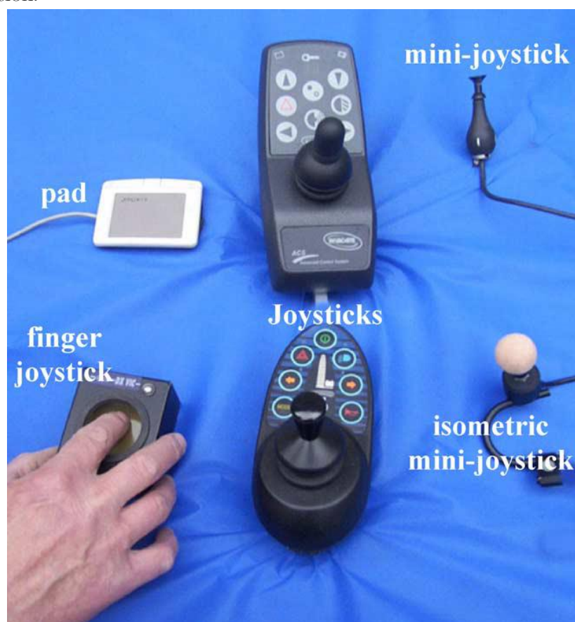
FIGURE II-18 : A COLLECTION OF STEERING DEVICES FOR NEUROMUSCULAR PEOPLE, USED BY PELLEGRINI ET AL. (2004)
