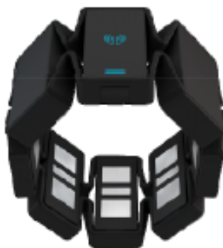
FIGURE II-12 : THALMIC LABS EMG BRACELET (MYO) 18
