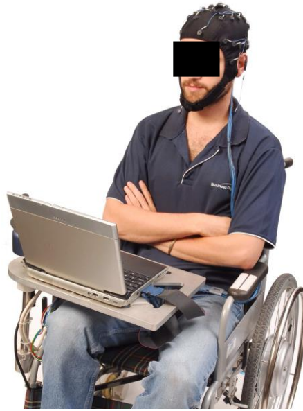
FIGURE II-16 : USER CONTROLLING A WHEELCHAIR WITH EEG HELMET (REBSAMEN ET AL. 2007)
