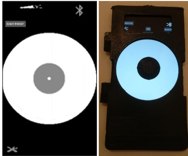
FIGURE III-18 : LEFT: THE SECOND PROTOTYPE OF THE TACTILE STEERING CIRCLE (WITH CONTINUOUS CONTROL), RIGHT: THE SECOND DESIGN OF THE PASSIVE HAPTIC FEEDBACK
