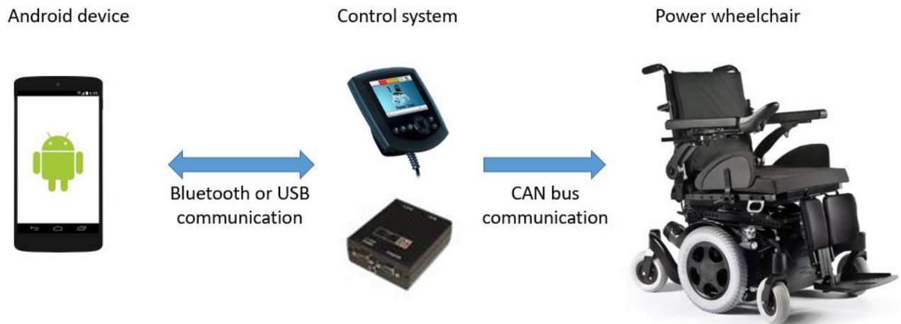
FIGURE III-11: COMMUNICATION SCHEMATIC OF WHEELCHAIR STEERING INPUT
