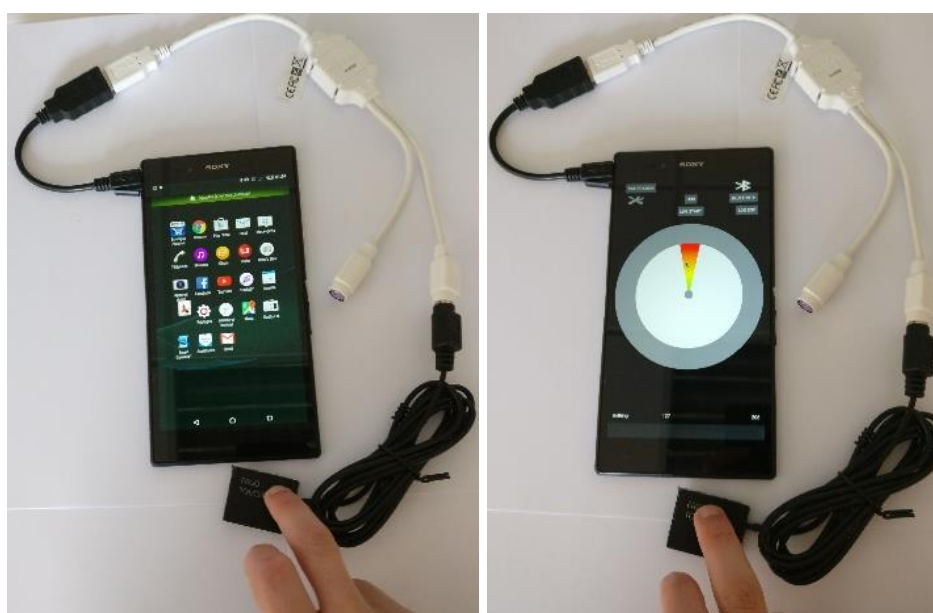
FIGURE VI-10 : A USER INTERACTING USING AN EXTERNAL SENSITIVE TOUCHPAD TO INTERACT WITH: THE APPLICATION LIST (LEFT) AND THE WHEELCHAIR STEERING APPLICATION (RIGHT).
