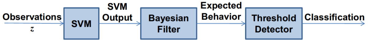
Figure 2.16 Stopping intent classifier using SVM and Bayesian Filter, after [64]
