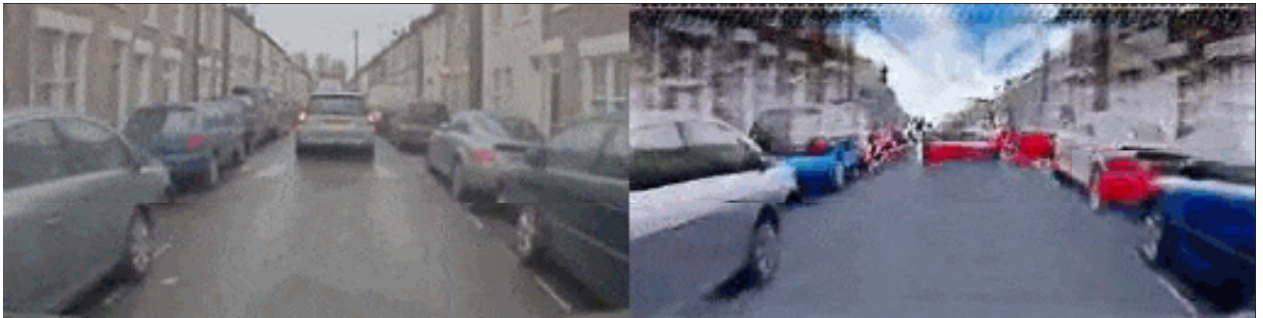
Figure 2.22 (a) Process flow of an end-to-end system for training and deployment, (b) images used by the network to decide with real perceived images (left) and the image transferred into the simulation space, after [101]
