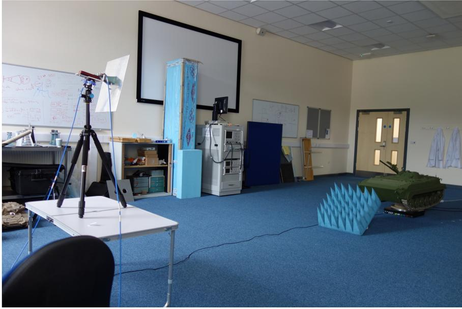
Fig. 2.9: Experimental setup. Some RAM is placed in front of the turntable to limit the unwanted returns from the turntable.
