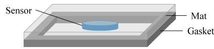
Figure 3.3: Example of a piezoresistive floor system. When a force stresses the material, its resistance decreases.
