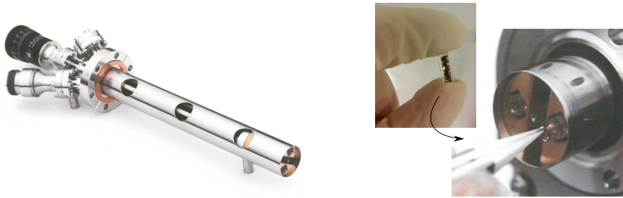
Figure II.5: Kentax two-cell molecular evaporator. The crucible is filled with molecules and inserted in the molecular evaporator. Left and right images were taken from the user manual provided by Kentax [133].
