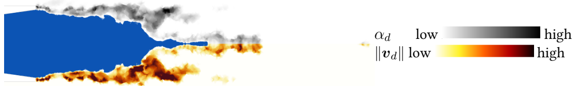
FIGURE 5.7: NIR7eq with atomization at t_{sim} = 2.5 t_{conv} on the slice at \theta = \pi/6 – blue isovolume of \alpha_2 = 0.99 , volume fraction of droplets \alpha_d , slip velocity norm \|\mathbf{v}_d\| .
