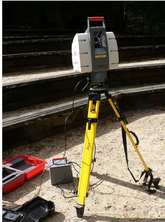
Figure 2.5 – Illustration of a TLS coupled to a GPS. Courtesy of Wikipedia Commons.
