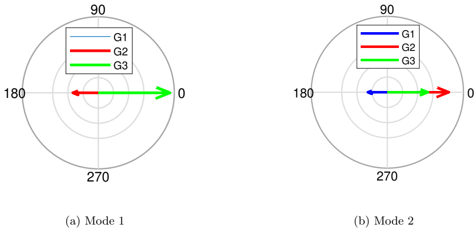
Figure 2.2 – Mode shapes for the two oscillatory modes
