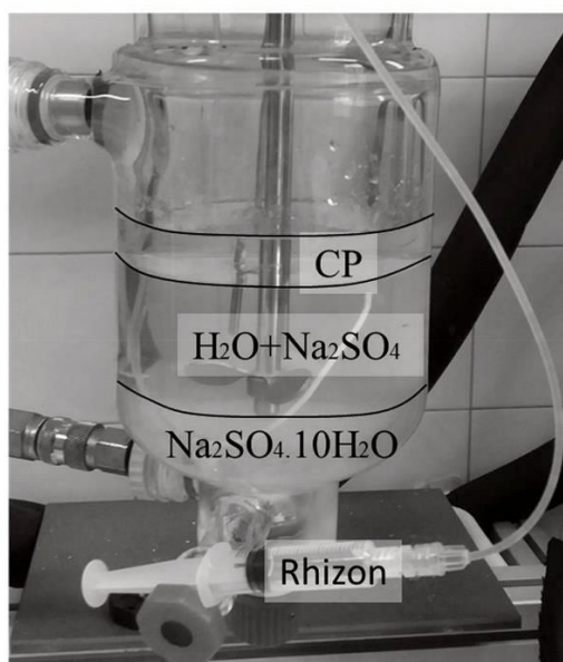
Figure 4. Photo of the experiment with \text{Na}_2\text{SO}_4 at 8%, 5.4 °C following the slow procedure.
