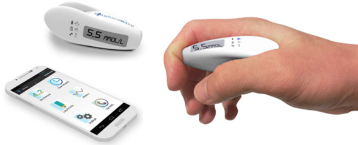
Figure 1.5: Glucowise TM - non-invasive medical device for glucose level detection [38]
