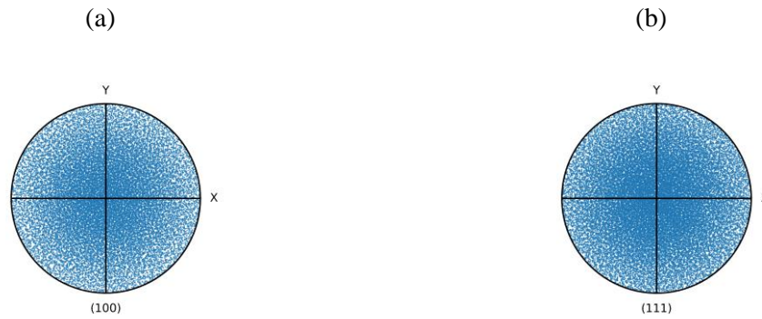
Figure IV-2: Pole figures of (a) 100, (b) 111 orientation for the crystallographic orientations implanted in numerical models
