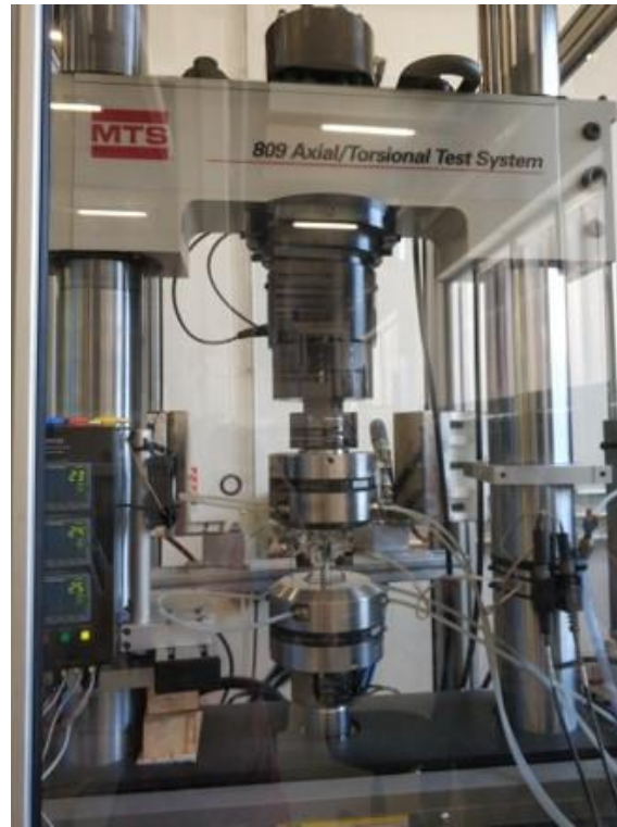
Figure II-29: Machined used in tensile test (MTS 809)
