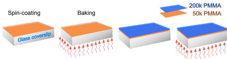
**Fig. 2.3.1.** Schematic representation of the spin-coating process for a double layer of PMMA.
