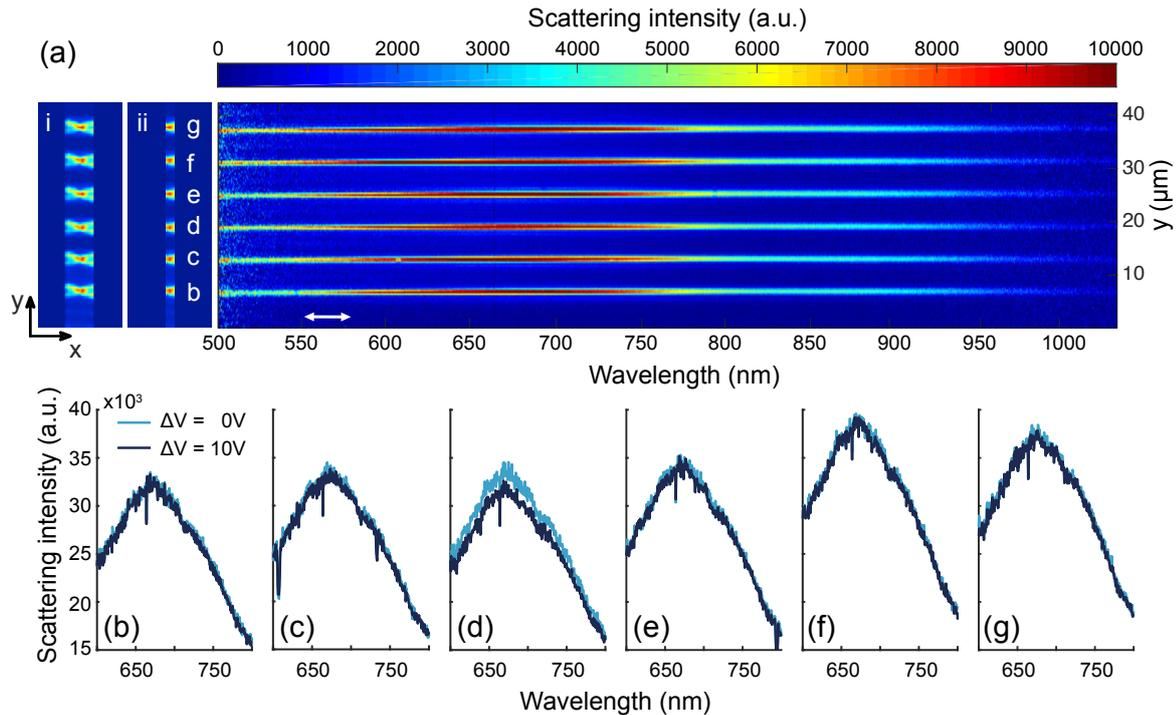
**Fig. 2.6.2.** Three dimensional spectrogram showing the dark-field spectra of six nanoantennas. The double arrow at the bottom left corner indicates the incident light polarization. Frames i and ii show the real image of the studied nanoantennas when the diffraction grating is at zero-order. (b,c,d,e,f,g) Corresponding binned spectra for every nanoantenna in (a).
