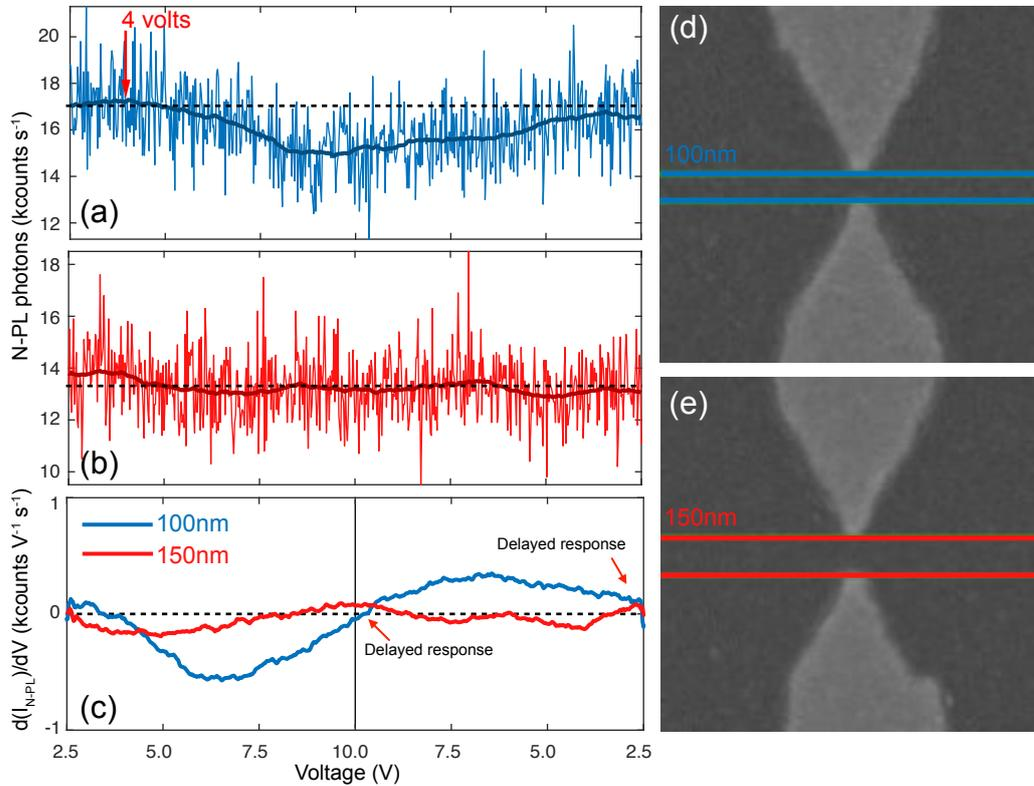
**Fig. 2.4.1.** Recorded N-PL in the gap region as a function of the applied voltage for nanoantennas with (a)  $\approx 100$ nm and (b)  $\approx 150$ nm gaps. (c) Change rate of the N-PL with the voltage applied. (d,e) SEM micrographs of typical studied nanoantennas with gaps similar to (a) and (b). The dotted lines indicate the zero bias N-PL in (a) and (b) and the zero N-PL change rate in (c)
