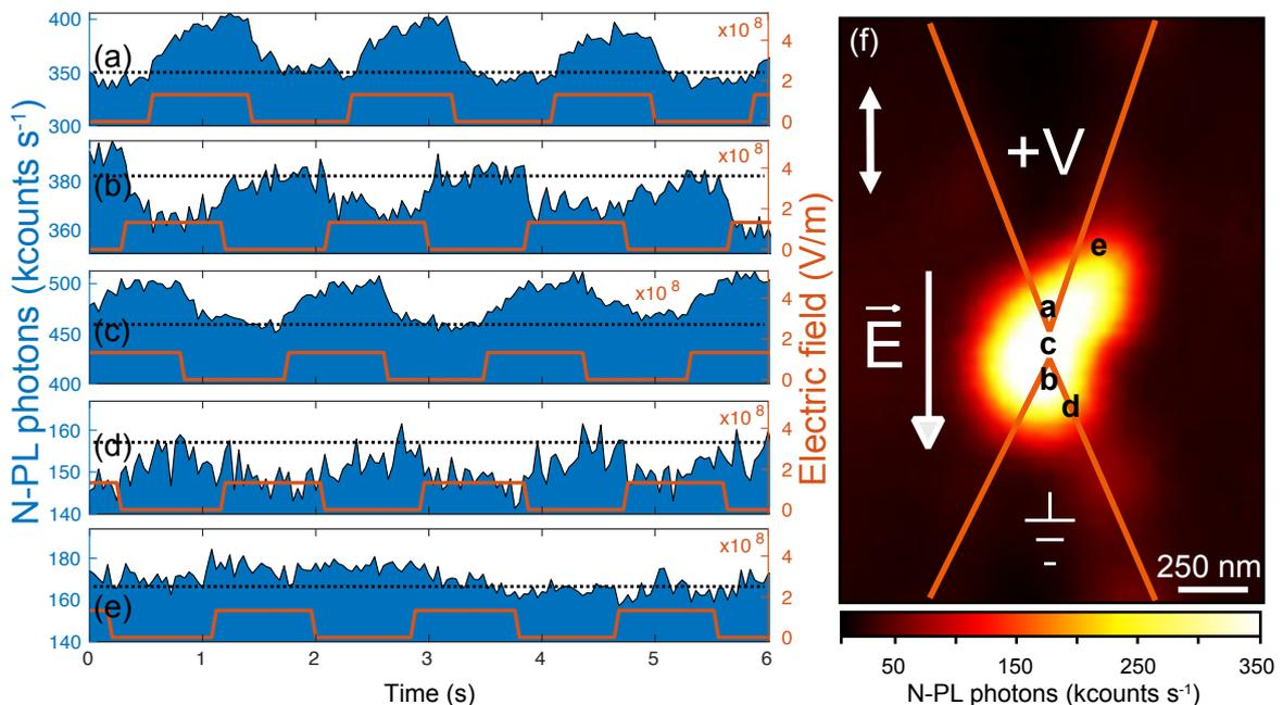
**Fig. 2.4.4.** (a,b,c,d,e) Corresponding time traces of the N-PL for each marked position in (b). The horizontal dashed line showing the approximated OFF state of the N-PL emission. (f) Confocal map of the N-PL emission of a 75 nm gap nanoantenna. The nanostructure is traced with orange lines. Each excitation point (laser tip position) is indicated with letters. The incident laser polarization is indicated by the double arrow.
