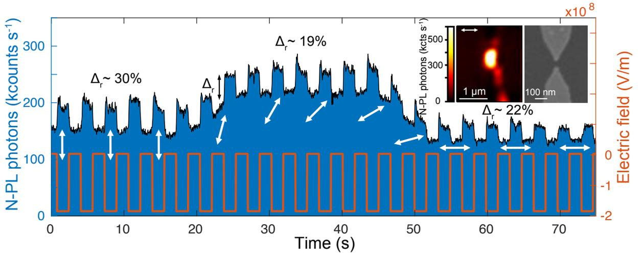
**Fig. 2.4.11.** Time trace of the recorded N-PL under the action of a 20 V squared electric signal for different incident laser polarizations. The relative modulation depth is pointed out as  $\Delta_{N-PL}$ . The white arrows show the polarization state with respect to the nanoantenna shown in the inset at that specific time. An N-PL confocal map and a SEM micrograph of the nanoantenna are shown in the inset.
