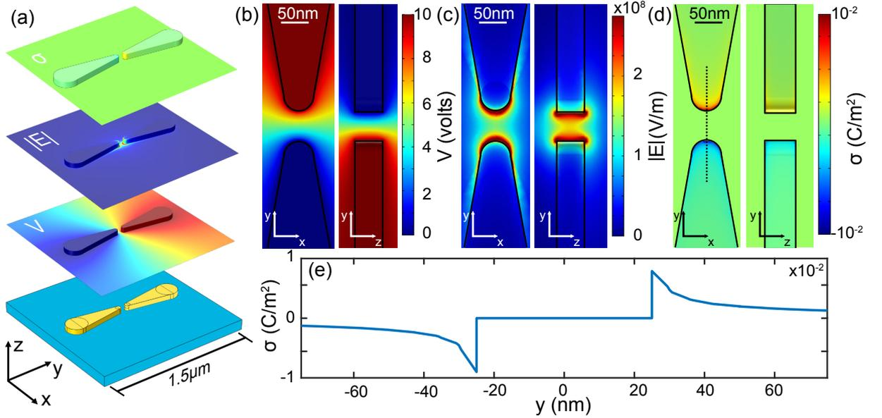
**Fig. 2.4.6.** COMSOL Multiphysics<sup>®</sup> simulation of a nanocapacitor with shape and dimensions similar to the studied nanoantennas. (a) Model configuration and different performed calculations. Electric (b) potential, (c) field and (d) surface charge density distribution in the gap region of the nanocapacitor. (e) Surface charge density along the dotted line indicated in (d).
