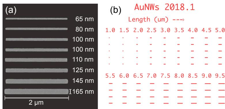
**Fig. 3.2.1.** (a) SEM micrographs of AuNWs showing the effect of the e-beam dose on the nanowire widths. (b) CAD design used to expose the resist and finally fabricate the AuNWs with different lengths.
