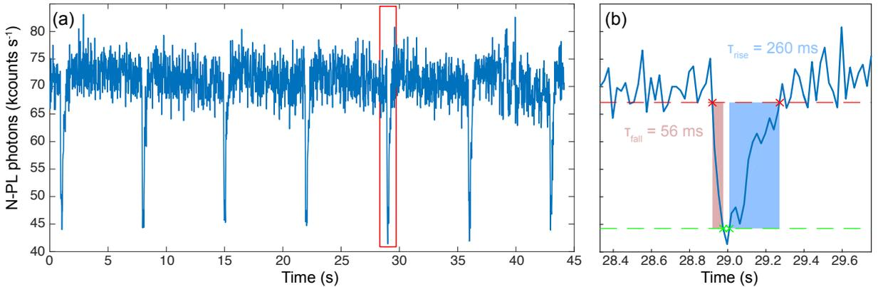
**Fig. 2.4.9.** (a) time trace of the emitted N-PL of a nanoantenna under the action of 8 V and 200 ms pulses. (b) Rise (blue-shaded area) and fall (red-shaded areas) times measured on a highly time-resolved trace of the N-PL indicated by the red square on (a). The red and green crosses indicate the referential points for the high and low values of the N-PL respectively.
