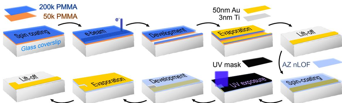
**Fig. 2.3.2.** Schematic representation of the complete fabrication process of the plasmonic device. A combination of e-beam and UV lithography defines a set of nanoantennas and the connecting electrodes respectively.
