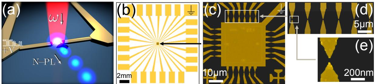
**Fig. 2.2.2.** Electrically controlled plasmonic device. (a) Schematic representation of the device operation. Two gold electrodes are separated by a nanometric gap to form an optical gap antenna. A femtosecond laser excites the structure and generates N-PL which is modulated by an applied electric field across the gap. (b) Real graphic representation of the plasmonic device. SEM micrographs of (c) all the nanoantennas, (d) zoomed at the top 6 nanoantennas and (e) a single nanoantenna.
