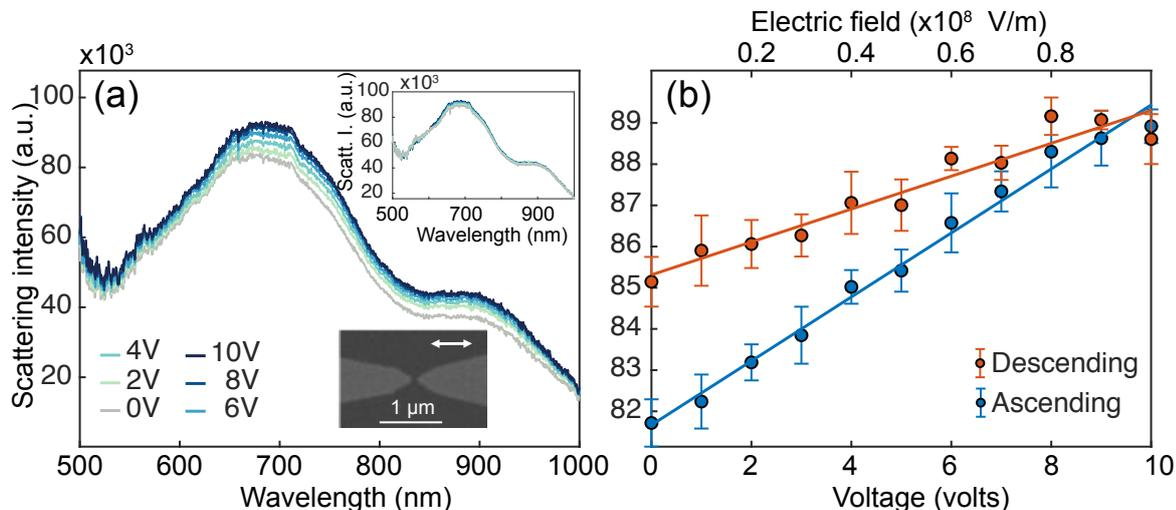
**Fig. 2.6.1.** (a) Dark-field spectra as the voltage across the gap of a bow-tie antenna is ramped-up. The insets show a SEM micrograph of the nanoantenna and the spectra for the subsequent ramping down. (b) Cross-section at  $\lambda = 650$  nm of (a).
