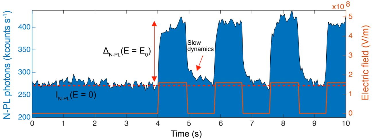
**Fig. 2.4.2.** In blue, the time trace of the N-PL emission (left ordinate axis) for a  $75 \text{ nm}$  gap nanoantenna. In orange, the applied squared electrical signal (right ordinate axis). The red dashed line and the double red arrow indicate approximately the values of  $I_{N-PL}(E = 0)$  and  $\Delta_{N-PL}(E = E_0)$  respectively.
