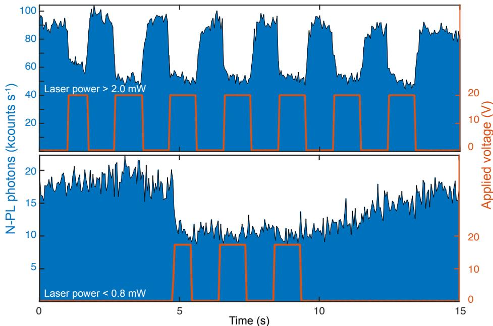
**Fig. 2.4.10.** N-PL time trace of an optical antenna for two incident laser powers and under the action of a squared time-varying voltage function with an amplitude of 20 V and a period  $T = 2 \text{ s}$ .
