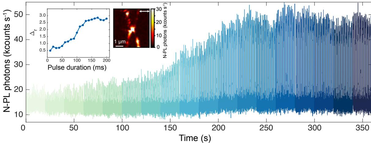
**Fig. 2.4.7.** Time trace of the recorded N-PL in a  $\approx 80 \text{ nm}$  gap under the action of time-varying 10 V pulses. Each color represents a different electrical pulse duration starting at 30 ms and increasing in 10 ms steps until reaching 200 ms. The insets show the dependence of the N-PL modulation depth as a function of the pulse duration and a N-PL confocal map of the studied nanoantenna.
