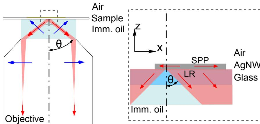
**Fig. 4.2.2.** SPPs are excited by a focused laser beam (not shown) and propagate through an AgNW. Leakage radiation (LR) is emitted under the phase-match angle range represented by  $\theta$ . An oil-immersion objective collects the leakage radiation. The transversal polarization is indicated by the blue arrows. The zoomed area corresponds to the dashed square. Schematic inspired by [285]
