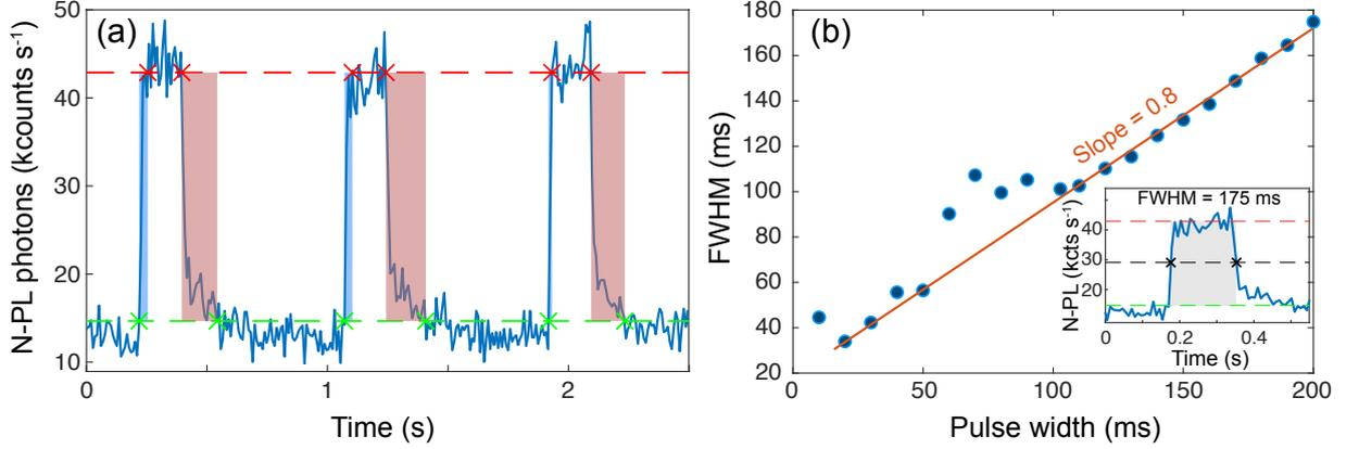
**Fig. 2.4.8.** (a) Rise (blue-shaded area) and fall (red-shaded areas) times measured on a highly time-resolved trace of the N-PL under the action of 10 V and 200 ms pulses. The red and green crosses indicate the referential points for the high and low values of the N-PL respectively. (b) Evolution of the FWHM of the N-PL pulses with the electric pulse duration. The inset shows the measured points for an N-PL pulse under the action of a 200 ms and 10 V pulse.
