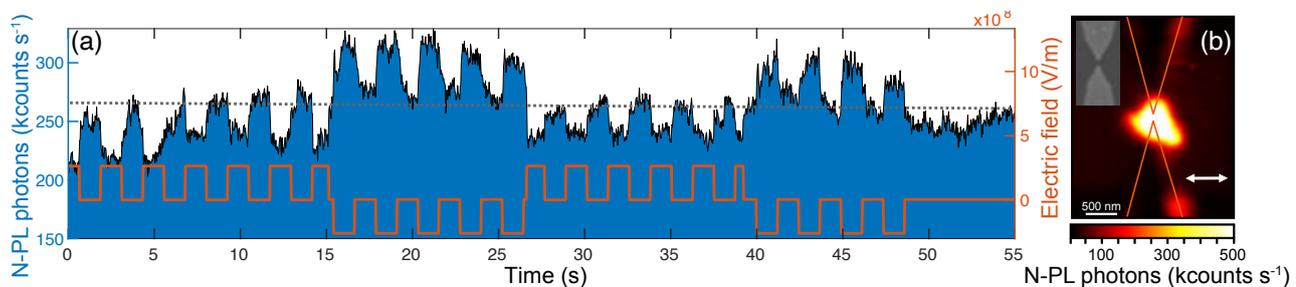
**Fig. 2.4.5.** Effect of the electric field polarity inversion on the recorded N-PL emission in the gap of a bow-tie antenna (100 nm gap). (a) Time trace of the N-PL and the electric signal. The dotted horizontal line refers to the no bias state. (b) N-PL confocal map of the nanoantenna. The inset shows an SEM micrograph of the antenna. The double arrow indicates the incident laser polarization.
