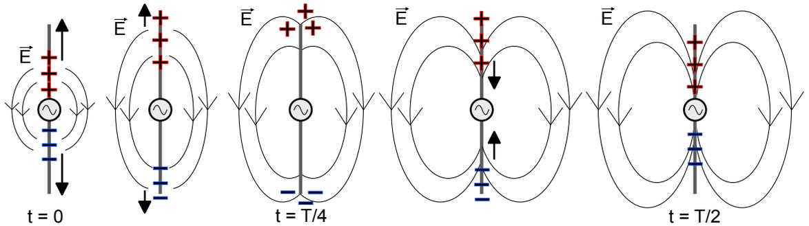
**Fig. 1.2.1.** Charge oscillations on a dipole as a function of time. In the case of an electric dipole, the driving current is supplied externally in the circuit. For optical antennas, the oscillations are generated by the incident EM field. Inspired by [55].
