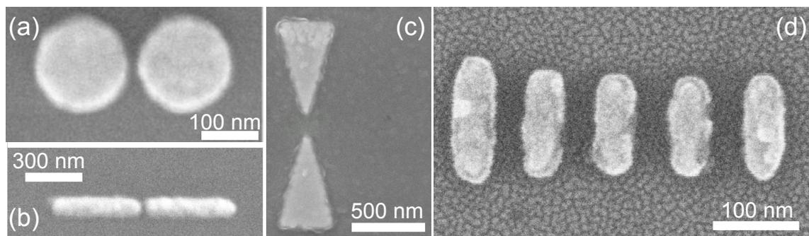
**Fig. 1.2.3.** Scanning electron micrographs of different optical antenna designs. (a) Hertzian dimer antenna. Reprinted with permission from [79]. Copyright 2012 American Chemical Society. (b) Dipole antenna. Reprinted with permission from [80]. Copyright 2008 by the American Physical Society. (c) Bowtie antenna and (d) Yagi-Uda antenna. SEM image courtesy of Xiao Yu, PhD student at the ICB lab.
