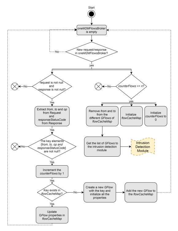
Figure 4.3: Workflow of the oneM2M features extraction module
