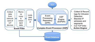
Figure 2.2: CEP-based IDS architecture for IoT
