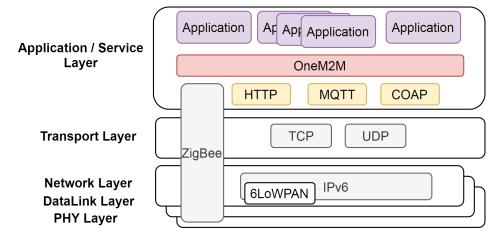
Figure 3.2: OneM2M service layer in the TCP/IP layer
