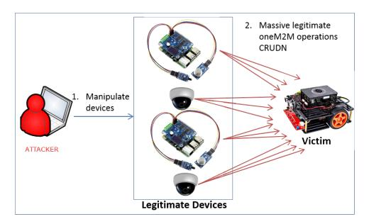
Figure 3.6: OneM2M flooding attack
