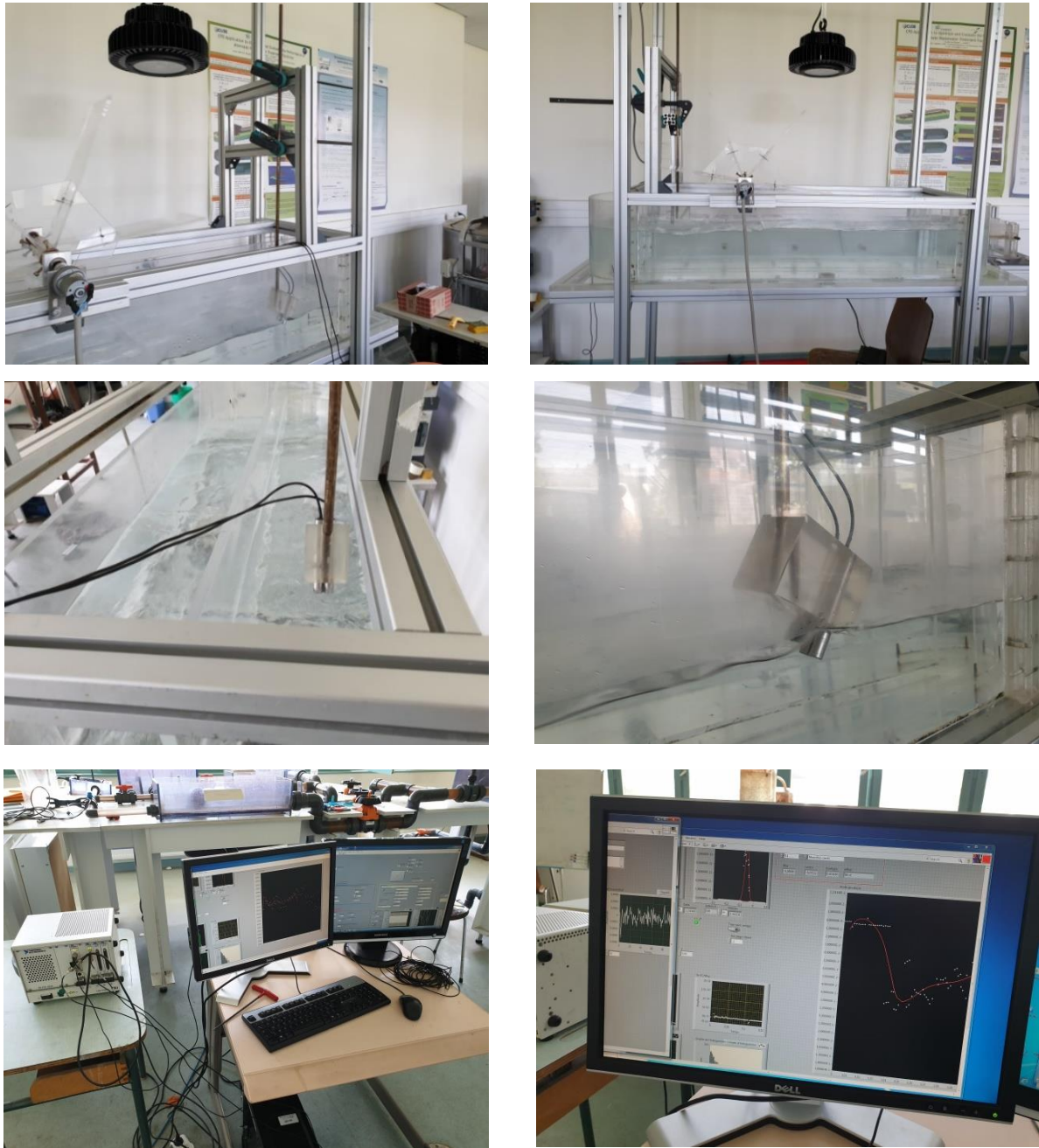
Figure 2.5- Transducer configuration and data accusation process layout during the experiment
