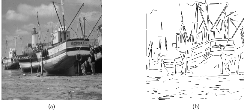
Figure 2.2: A line detection algorithm. In (a) we present the original image and in (b) a binary image. The black lines correspond to the lines detected by the LSD algorithm, see http://demo.ipol.im/demo/gjmr_line_segment_detector/ for an online demonstration.
