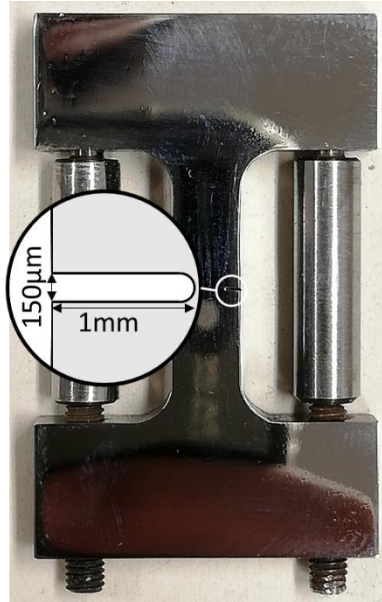
Figure 59 The specimen used to perform constant displacement test.
