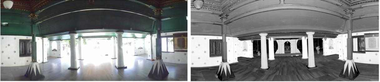
Figure 1.6: Example of a section of a panoramic image captured by the TLS. The left figure shows the RGB image, with strong overexposure due to sunray intensity. The right figure shows the intensity image, which was preferred in the tie point identification process.
