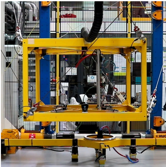
(a) Platform without cross (MPNC, 266 kg)
