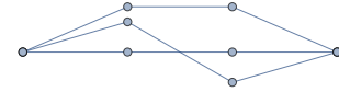
Figure 1.11: Here we represent the 2 bending modes of filament subdivided in 4 parts (the 2 remaining one are stretching modes). A system with N degrees of freedom has N normal modes. However two angular forcings in opposite directions at the ends of the system can enhance filament's mode 2 bending and will require at the very least 3 subedges to be possible.
