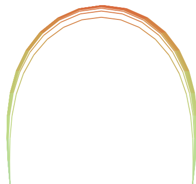
Figure 1.17: We display the geometry of an Euler elastic rod made of N = 20 edges. In red edges are compressed, in green they are at rest. For strong compression rates, we end up with a coupling between bending and stretching, even for large \mu .
