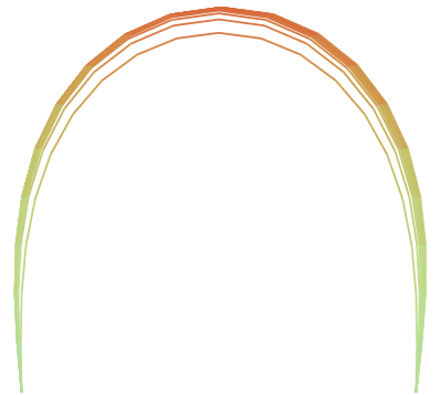
Figure 1.17: We display the geometry of an Euler elastic rod made of N = 20 edges. In red edges are compressed, in green they are at rest. For strong compression rates, we end up with a coupling between bending and stretching, even for large \mu .
