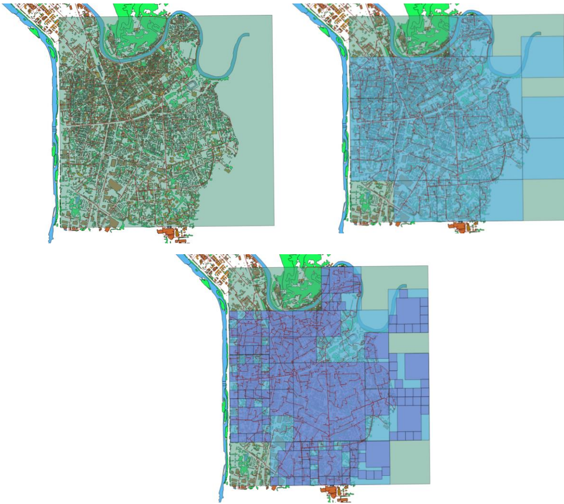
Figure 2: Iterations 1 and 2 of the fractal process to plan the power grid (upper left panel – generator ; upper right panel – initiator ; bottom panel – 2 nd iteration)
