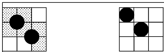
Figure 2-7: Illustration of the box counting method (left: random coverage / right: minimum coverage)
