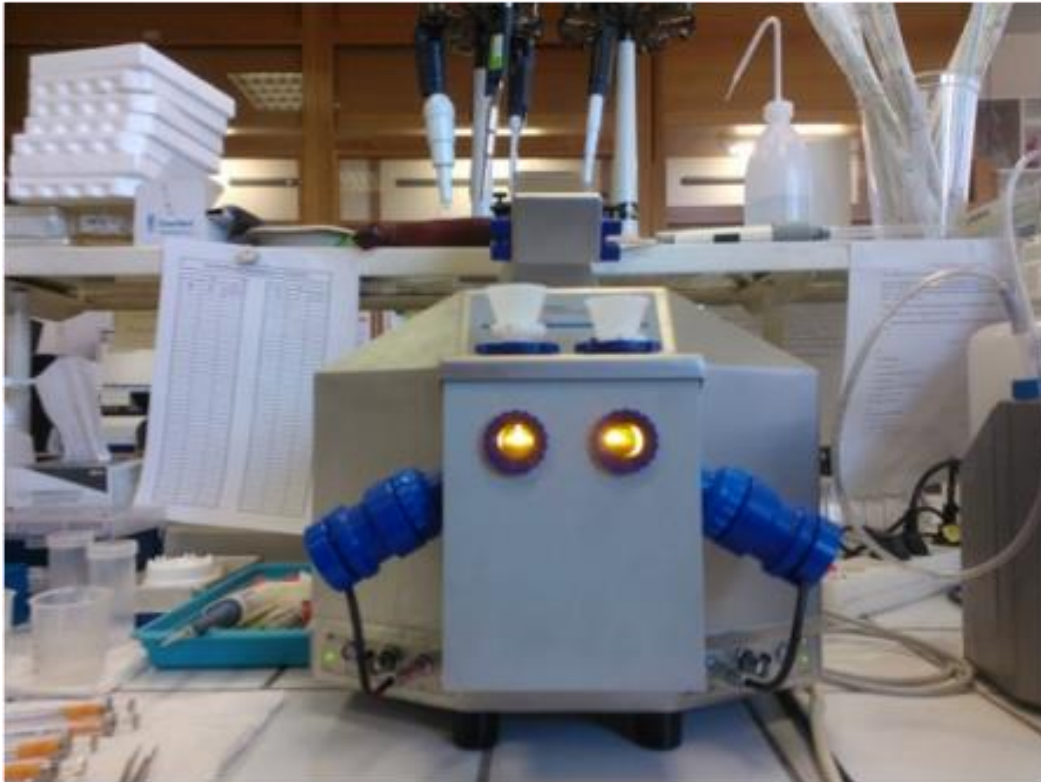
Figure 13. The oxygraph used for mitochondrial respiratory chain assessment.
