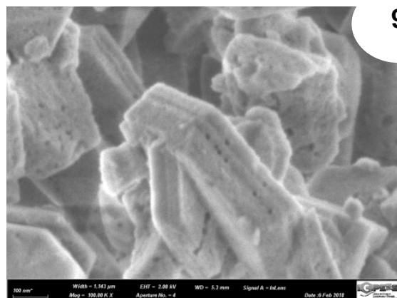
Figure SEM 9: Desilicated by with TPAOH and NaOH Y-zeolite D15
