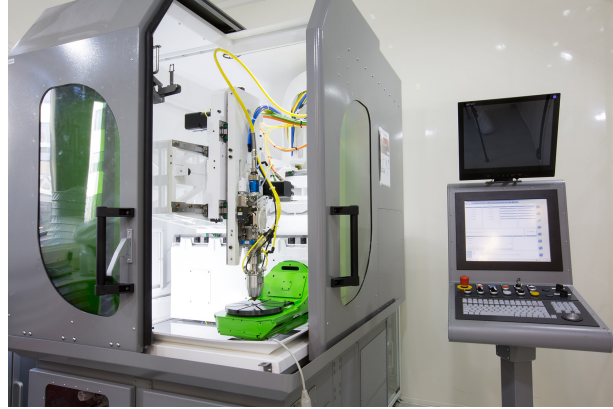
Figure 2.1: Photo of the DED machine at the Laboratoire de Mécanique des Solides of École Polytechnique .
