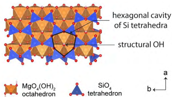
Figure 3. Hexagonal rings of Si tetrahedra with structural OH groups in the centers.
