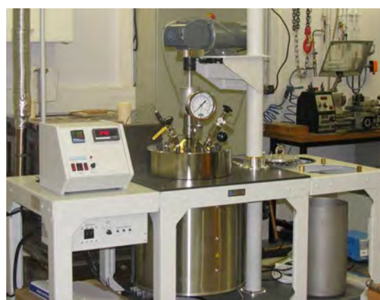
Figure 5. An 18.5 L stainless steel autoclave used for the preparation of P3-nanotalc (GET laboratory, Toulouse, France; Parr Instrument Company; property of Imerys Talc Europe).
