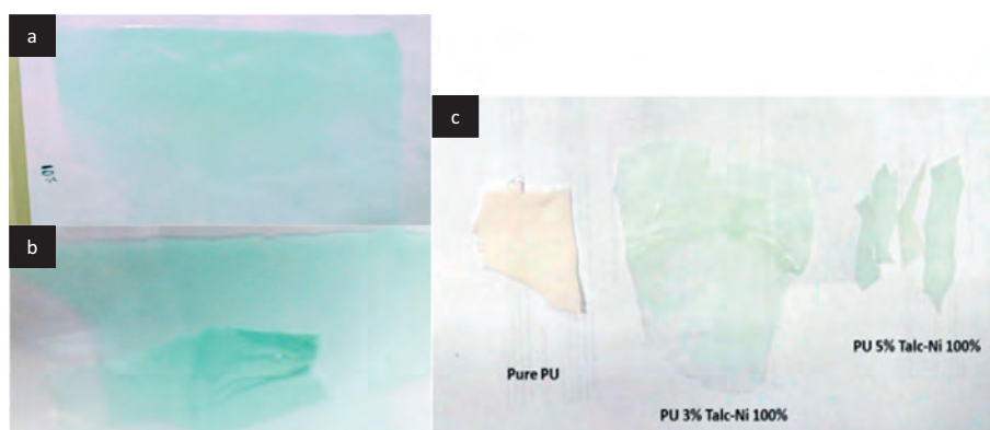
Fig. 19. Polyurethane films with various Ni-bearing talc contents: a) homogeneous distribution of nano-charges; b) heterogeneous distribution of nano-charges; c) films containing low talc charge.
