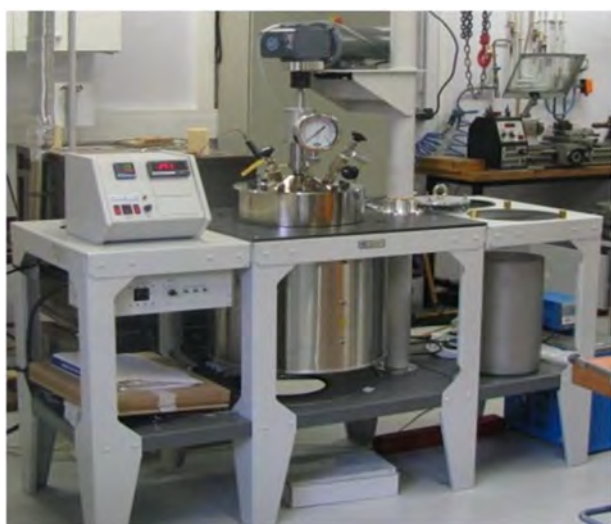
Fig. 3. 18 L batch reactor implanted at GET and owned by IMERYs.
