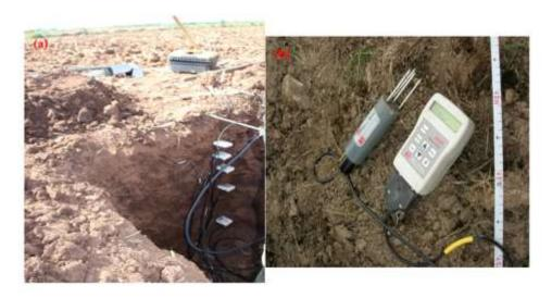
$\textbf{\it Figure III. 4.} \ Photograph \ of \ (a) \ TDR \ (Time \ Domain \ Reflectometry) \ and \ (b) \ Theta \ Probe \ instruments$
