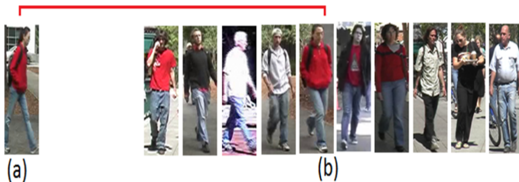
Figure 3.1: Image (a) is the Test Image, (b) are the images of the gallery set with sorted order. The feature vector used is the RGB channel values and its gradients. For the similarity score we calculated the distance between the covariance matrices.
