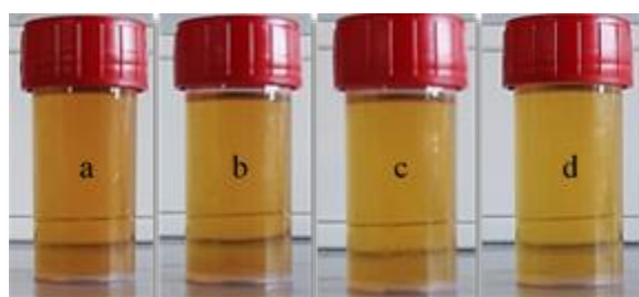
Figure 4 - Permeates after ultrafiltration of feed juice with a) 150 kDa b) 20 kDa c) 10 kDa d) 5 kDa PES membranes. Ultrafiltration was done at the pressure of 3 bar, and under the stirring at 400 rpm.
