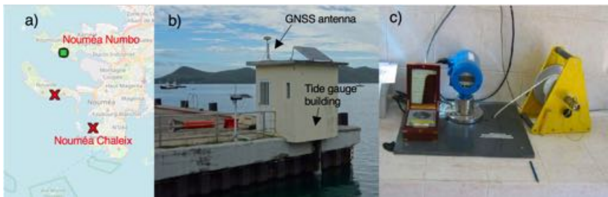
Figure 3.4: Location of the Nouméa tide gauge (a, b) and GPS station (b), and the tide gauge inside the building. Source: Refmar 2017, SONEL 2017.
