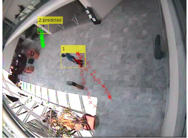
Figure IV-27: Object 2 exiting the scene “LeftBox”, at the frame 238.
