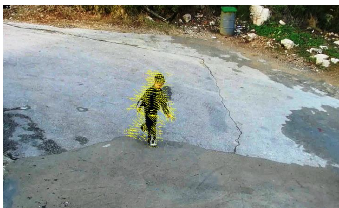
Figure III-6: Walking Scene: Uniformity Filtering result (regular size) of Figure III-5-c; we can notice that the groups of false vectors on the left and near the boy are deleted.
