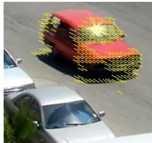
Figure III-10: Highway 4 scene: Texture Filtering result (zoomed size) of Figure III-9; we can notice that the false vectors near right doors of the car are deleted
