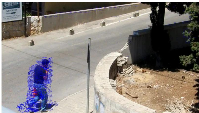
Figure III-4: Scene with a person (Frame 25): Marzat's algorithm applied for estimating motion.
