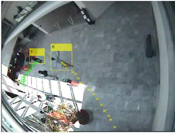
Figure IV-32: Objects distant interaction in the scene “Fight_RunAway2”: frame 279 showing the trajectories of each object, and the distant aggressive interaction between objects 1 (showing as 5) and 2 (showing as 6).
