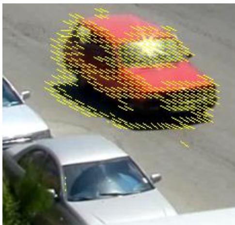
Figure III-9: Highway 4 scene: Uniformity Filtering result (zoomed size) of Figure III-8-c; we can notice that the false vectors around the car are deleted.
