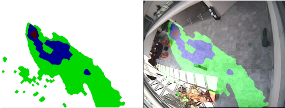
Figure IV-14: Figure showing the routes in green and the 2 levels of activity hot spots in blue and red, of scene "LeftBox".
