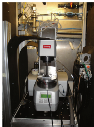
Figure 3.27 – In situ Rheo-reflectometry on FIGARO from reference [138]
