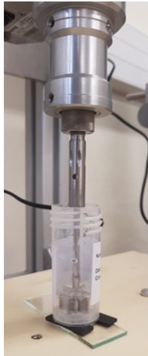
Figure 3.14 – Mixing and homogenization of the PTR2 gel sample by slow rotations with a rotary rheometer with blades.
