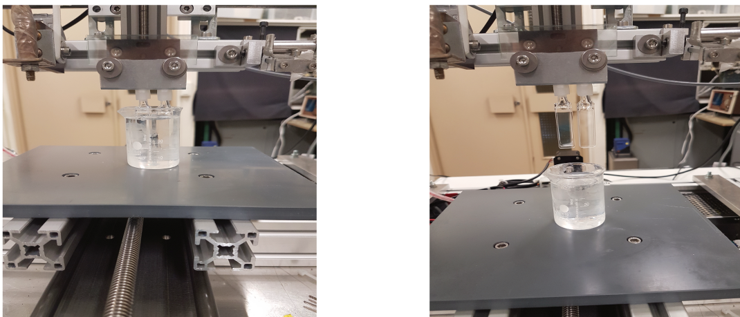
Figure 3.22 – Dip coating, immersion stage (left) and drying stage (right)
