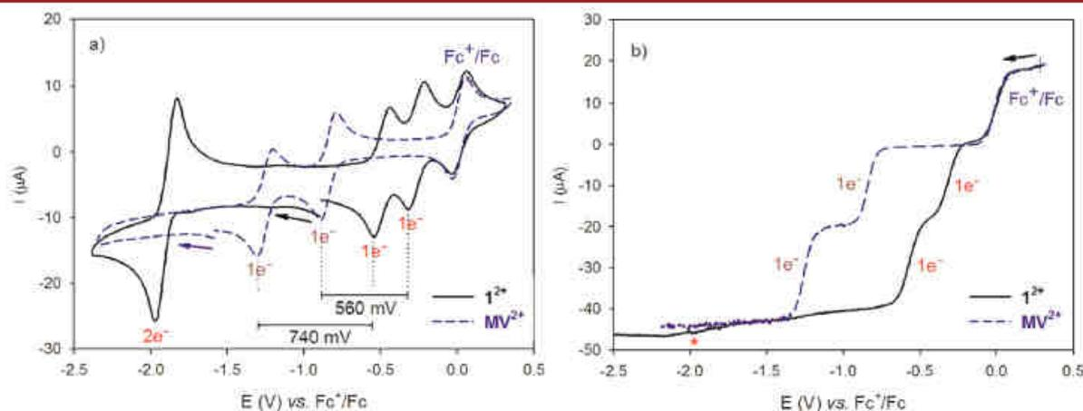
Figure 2. CV (a) and rotating disk electrode voltammetry (b) of **1**<sup>2+</sup> and MV<sup>2+</sup> in CH<sub>3</sub>CN + 0.1 M TBAPF<sub>6</sub>; working electrode = glassy carbon, pseudoreference = Pt, counter electrode = Pt, internal reference = Fc. (a)  $\nu = 0.1$  V/s; (b)  $\nu = 0.02$  V/s, rotation: 1000 rpm.
