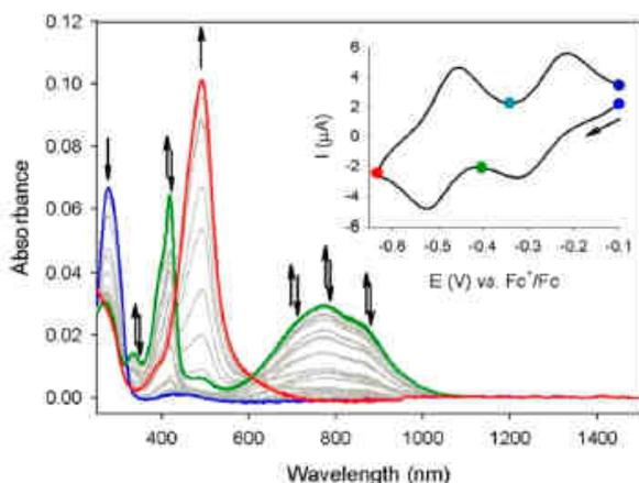
**Figure 4.** UV-Vis-NIR monitoring of the reduction of  $1^{2+}$ . (inset) Corresponding CV at scan rate of  $0.01 \text{ V s}^{-1}$ . Solution ( $c = 1 \times 10^{-3} \text{ M}$ ) of  $1^{2+}$  in  $\text{CH}_3\text{CN} + 0.1 \text{ M TBAPF}_6$  recorded with an optically transparent thin-layer (0.2 mm) electrochemical cell equipped with an Au mini-grid WE and  $\text{CaF}_2$  optical windows, reference  $\text{AgCl}/\text{Ag}$ .
