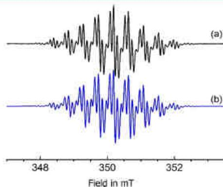
**Figure 5.** X-band EPR spectrum of  $1^{1+}$  (a) in  $\text{CH}_3\text{CN}$  at  $10^{-3} \text{ M}$  at room temperature; (b) simulated spectrum.
