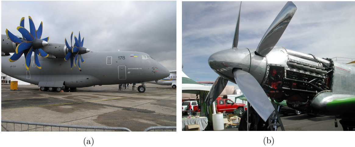
FIGURE 1.6 – Application of counter-rotating system on aircraft (a) Antonov AN-70 (Paris Air show 2013) and (b) P51 of North-American ( Source:wikipedia.org )
