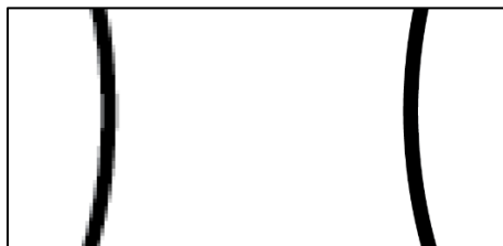
Figure 39: Pixelization; the enlarged curve on the left represents Raster the other represents Vector
