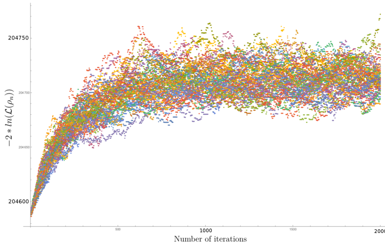
Figure 5.22: Exploration of the likelihood space of \hat{\rho}_{-|0}^{exp} starting from \hat{\rho}_{-|0}^{ML} for 50 different beginnings of the Metropolis-Hastings algorithm. The thermalization is considered to be reached after 1250 iterations.
