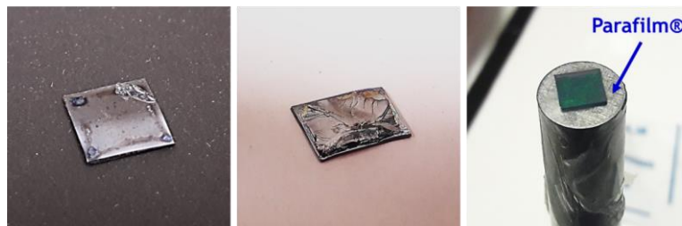
Figure 2-8. (Left-Middel) Examples of surfaces of PAA with broken pieces of macroscopic hydrogel after an alignment process in air without the Parafilm® protection. (Right) Hydrogel thin film glued to a stainless steel cylindrical probe and covered with a stretched layer of Parafilm®.
