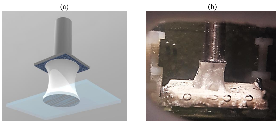
Figure 5-11. Underwater adhesion experiments. (a) Schematics and (b) Picture of the probe tack test performed underwater on a graft copolymer sample after a temperature switch at 50^{\circ}\text{C} in a medium at 0.75 M NaCl.
